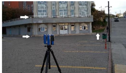
Figure 1. Placement of a reference sphere used as a registration target. From S. W. Nazari, M.S. thesis, 2020 [4].
