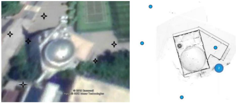
Figure 2. Positions of the eight scan stations around the Farabi Mosque before and after scanning. From S. W. Nazari, M.S. thesis, 2020 [4].
